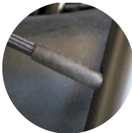
Rubber oversleeve stops wear.
